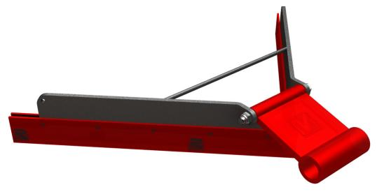
The PU 88 is a stable plough with steel frame and exchangeable PU-scraper strips. When fitting the plough, a tube of diameter 40 mm is threaded through the PU link. The tube is then fixed to the frame of the conveyor. The plough can be modified for reversible drive.
